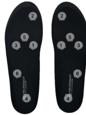
(a) The locations of six pressure sensors embedded within the insole. These sensors measure absolute pressure values at specific points on the foot.
